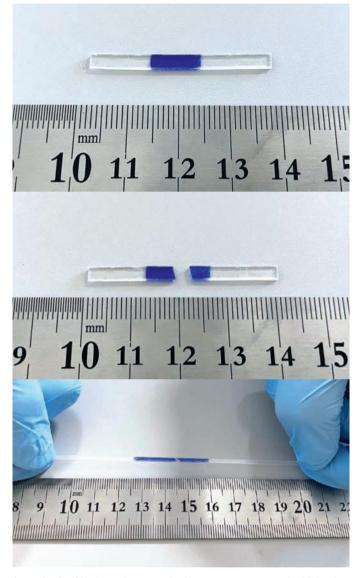
A sample of self-healing polyisoprene (top) was cut into two pieces (middle) and then pressed together for 15 seconds. After one minute, the sample could be stretched to more than double its original length without breaking (bottom).
