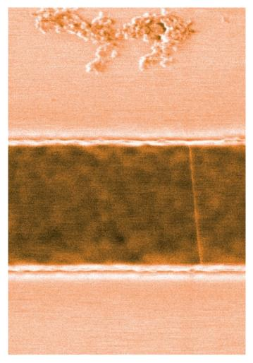
A carbon nanotube suspended across a trench in a silicon substrate. By developing a method that allows such suspended nanotubes to be functionalized with organic molecules, RIKEN researchers have enhanced their usefulness for sources of single photons.
