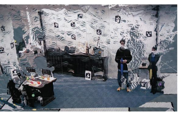
Task-oriented mobile robot, Butsukusa, autonomously patrols one of the GRP's rooms guided by a camera-and-laser system that helps it measure distance. It uses a deeplearning driven recognition module to identify objects, humans and the environment (above), as well as its location and speech. A combination of sensors that take in audio, visual and thermal information has been proposed to increase its ability to recognize people and their emotions.
