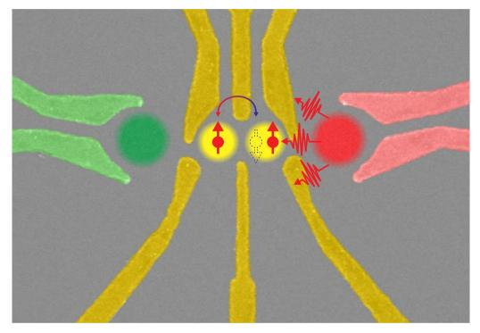
A double quantum dot device enables the study of how the spin and charge of an electron influences thermodynamic action in the presence of a lattice temperature gradient. Lattice vibrations known as phonons (three red squiggles) come from the quantum dot (colored red) on the right, which acts as a local heater. They can cause the spin on of the two electrons (yellow dots) to flip, which is detected by the quantum dot (colored green), which acts as a charge sensor.
